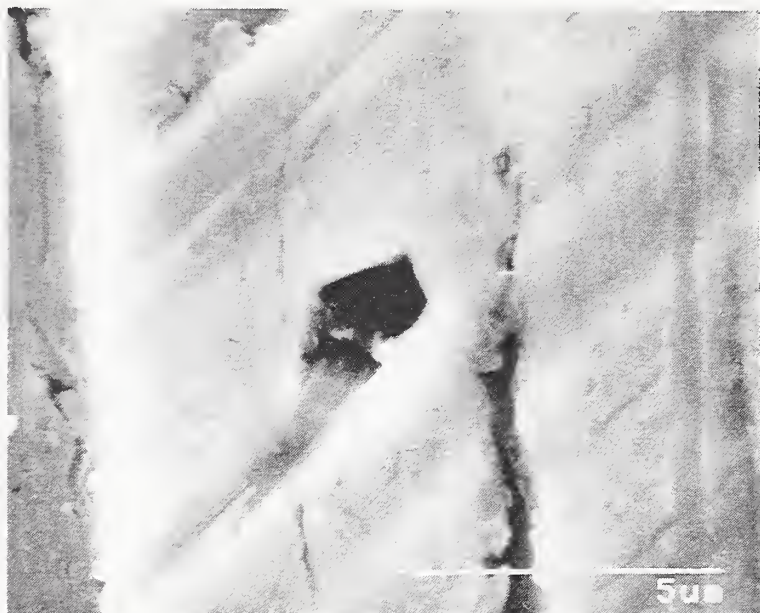
Fig. 31. SEM micrograph of \text{Al}_2\text{O}_3 particle embedded in 52100 steel disk.
